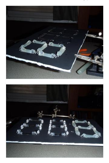
With all of the LEDs in place and the hot glue set, the final step was to add the colon. To do this, I made two larger holes to fit the entire LED body into. This kept the LEDs from standing too far off of the board and allowed a layer of glue coating to be placed over them as well. This thing is finally starting to look like something!
