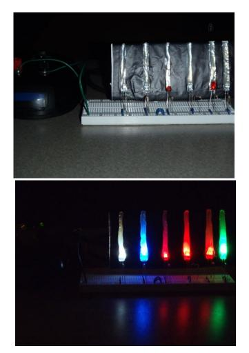
I finally settled on using a strip of aluminum foil glued to a black background. Two LEDs would be fixed at each end of the foil, and a coating of glue would be placed in a strip over the LEDs and foil to diffuse the light. I had originally planned on using red LEDs, but I liked the way the green ones looked. In my test setup, I only used one LED at a much higher current. The following table details the resulting LED electrical characteristics.
