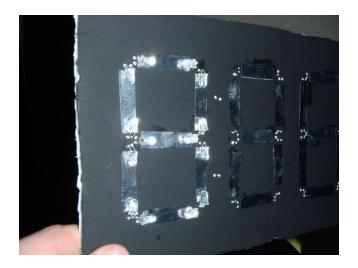
With all of the LEDs for one segment in place, a layer of hot glue was added. This was a bit messy, but I trim the edges later in the process. After the glue had set, a quick and successful test of each LED let me continue in the building process with confidence.
