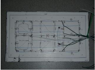
With a series resistance of  $560\Omega$  for each segment, a source voltage of 5V, and an LED forward voltage of 3V, each register pin should only be sourcing about 3.6mA [(5V - 3V) /  $560\Omega$ ]. Considering that each digit is only on 1/3 of the time because of the multiplexed control and each segment is comprised of two parallel LEDs, only about 0.6mA are flowing through any LED at any given time. With the diffusion, this is plenty enough to fully illuminate the display!
