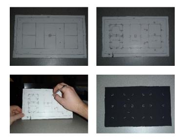
With the LED lead holes outlining the segment placement, I glued aluminum strips in place. These strips will serve as a reflective background for the light, aiding in the overall diffusion. Once the foil was set, I added all of the LEDs for the first digit.
